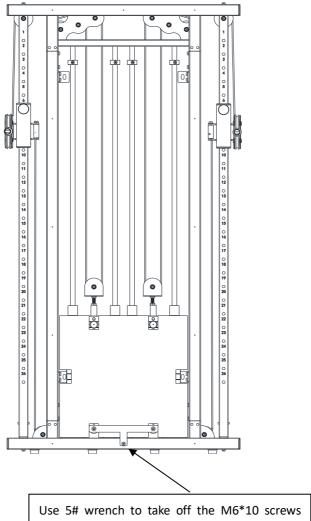
Use 5# wrench to take off the M6\*10 screws from the fixed plate.
