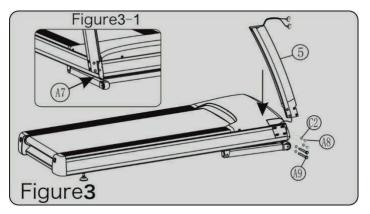
3.3 In upper outer side, using Bolt M10X160 (A7) that was assembled on frame to tighten.(Attention: bolt head position is the front underside. See Figure 3-1)
