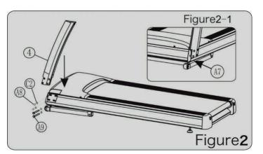
tighten.(Attention: bolt head position is the front underside. See Figure 2-1)
